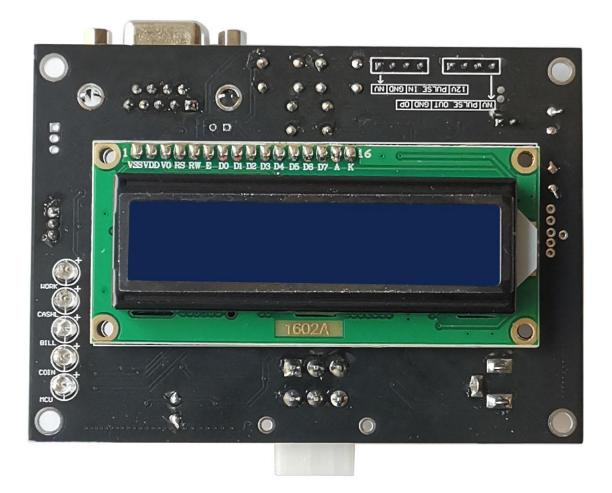
LCD panel on the front side to show device information and working status Five LED to show the payment device connected status
